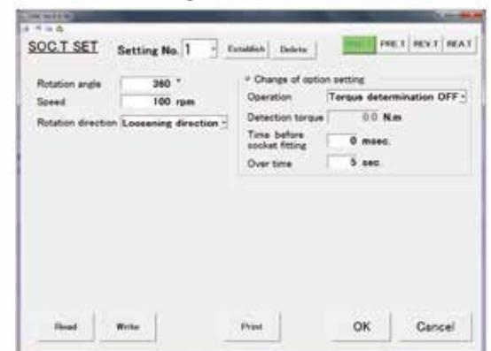
Screen for setting the rotation for matching a bolt with a socket.
