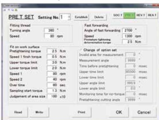
Screen for setting bolt setting status to seating. (temporary tightening)
